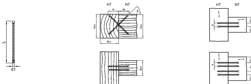
$a_2 = \text{min. } 40 \text{ mm}, a_{2c} = \text{min. } 24 \text{ mm}, k = \text{min. } 12 \text{ mm}$
